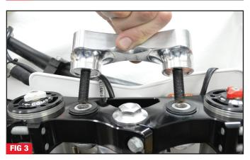
Center your handlebars in the lower handlebar mount and install the 2 top handlebar clamps. With the supplied 30mm bolts, using a 10mm socket torque the 4 top handlebar clamp bolts to the manufactures specifications (Fig 5).
